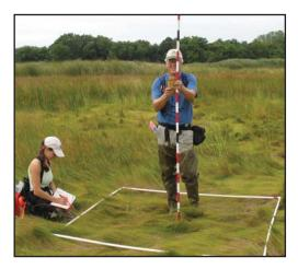
CLEAR researchers using a GPS receiver to determine the center of a field inventory site in the Ragged Rock Creek tidal marsh.
