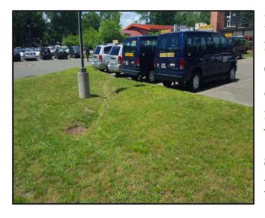
For this location, we recommend implementing a rain garden inside the barrier on the northeast side of the parking lot. The curb would be cut to allow access into the rain garden since the water flows naturally to the area. Also, the existing drain would be raised for the bypass system. In order to maintain safety it is recommended that the area be fenced in to prevent anyone from entering the garden.
