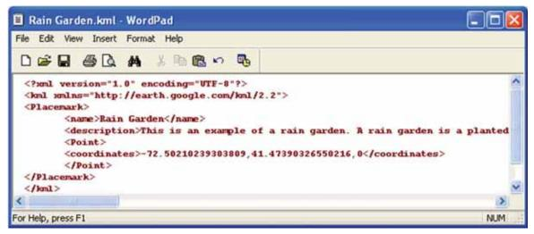
KML uses a simple tag-based structure with nested elements and attributes and is based on the XML standard
